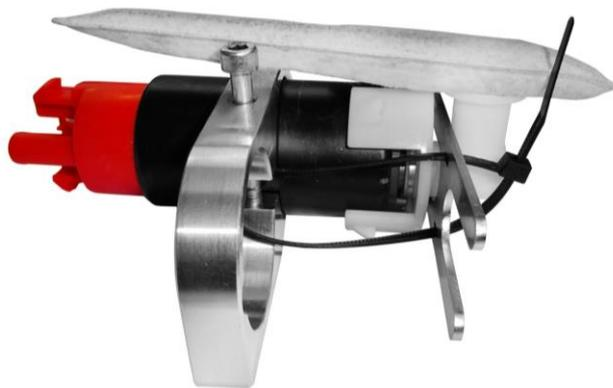
8. Refit the pre-filter sock to the pump - Install the pre-filter retaining plate to both pre filters and push home over the nose of the pump. There should be a small gap between the pump mount and the retaining clips on the pre-filter of 1-2mm. Tighten the zip tie on the plate evenly, A small wiggle on the zip tie may be required to even the tension on the plate
